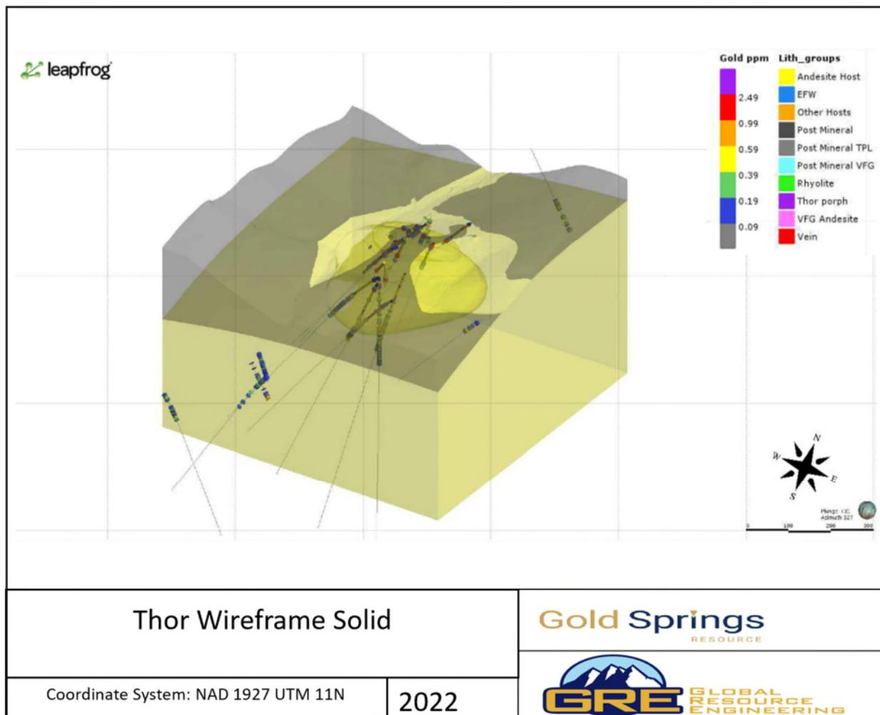
Using MicroModel, GRE modeled gold and silver grades into the Thor block model using ID2.5, OK, and NN interpolators. For each estimate, GRE first estimated the blocks only within the Mineralized Zone. Troy ounces of gold and silver contained were calculated from the modeled grades using the block specific gravity. GRE chose the ID2.5 method with 2 holes required as the preferred method because it had better local variability that more closely fit the data.
