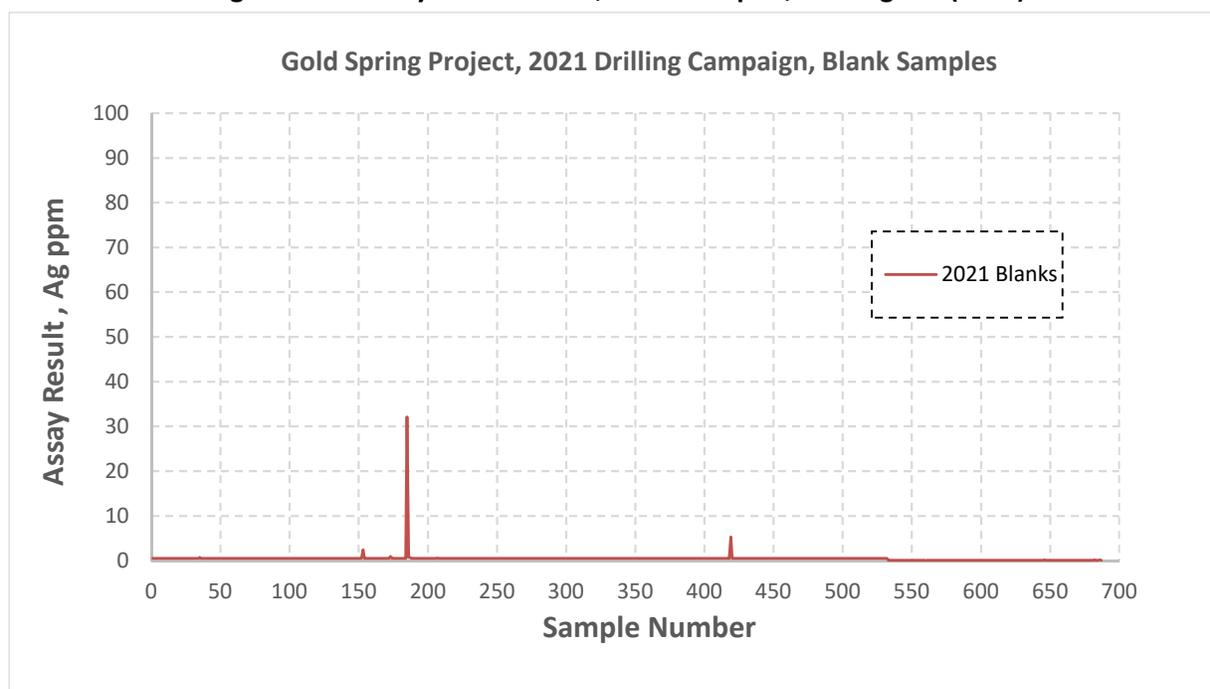
As a result, considering excursion rates of 1.45% and 1.16% for gold and silver, respectively, and that the values of these excursions were well below the probable lower limit of the cutoff grade of gold, the GRE QP believes the results indicate there is no artificially introduced contamination in the sampling preparation process that would materially affect a mineral resource estimate.
