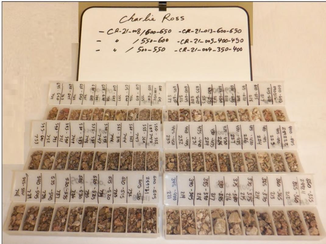
Photo 12-6: Ninety-Two RC Sample Chip Intervals in Chip Trays Selected from Seven Holes at Etna
