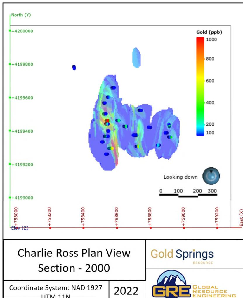
**Figure 14-36: Charlie Ross Section Composites and Block Model Cross Section**
