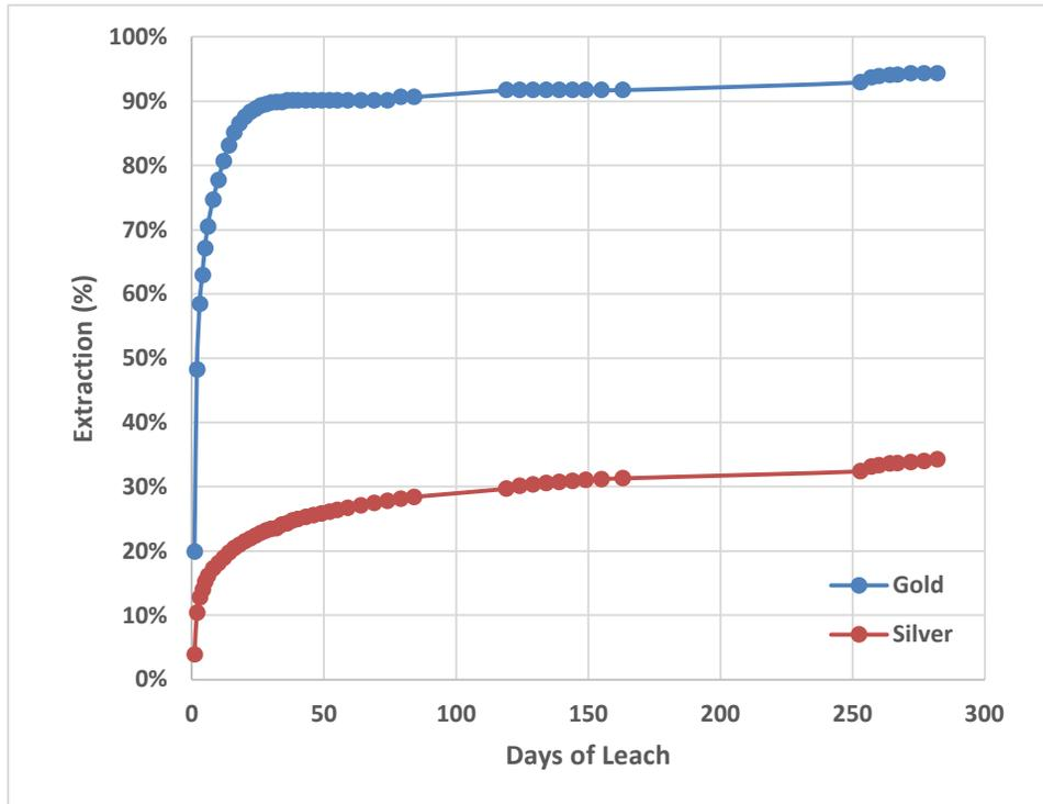
Figure 13-4: Jumbo Composite 2 Column Leach Results
