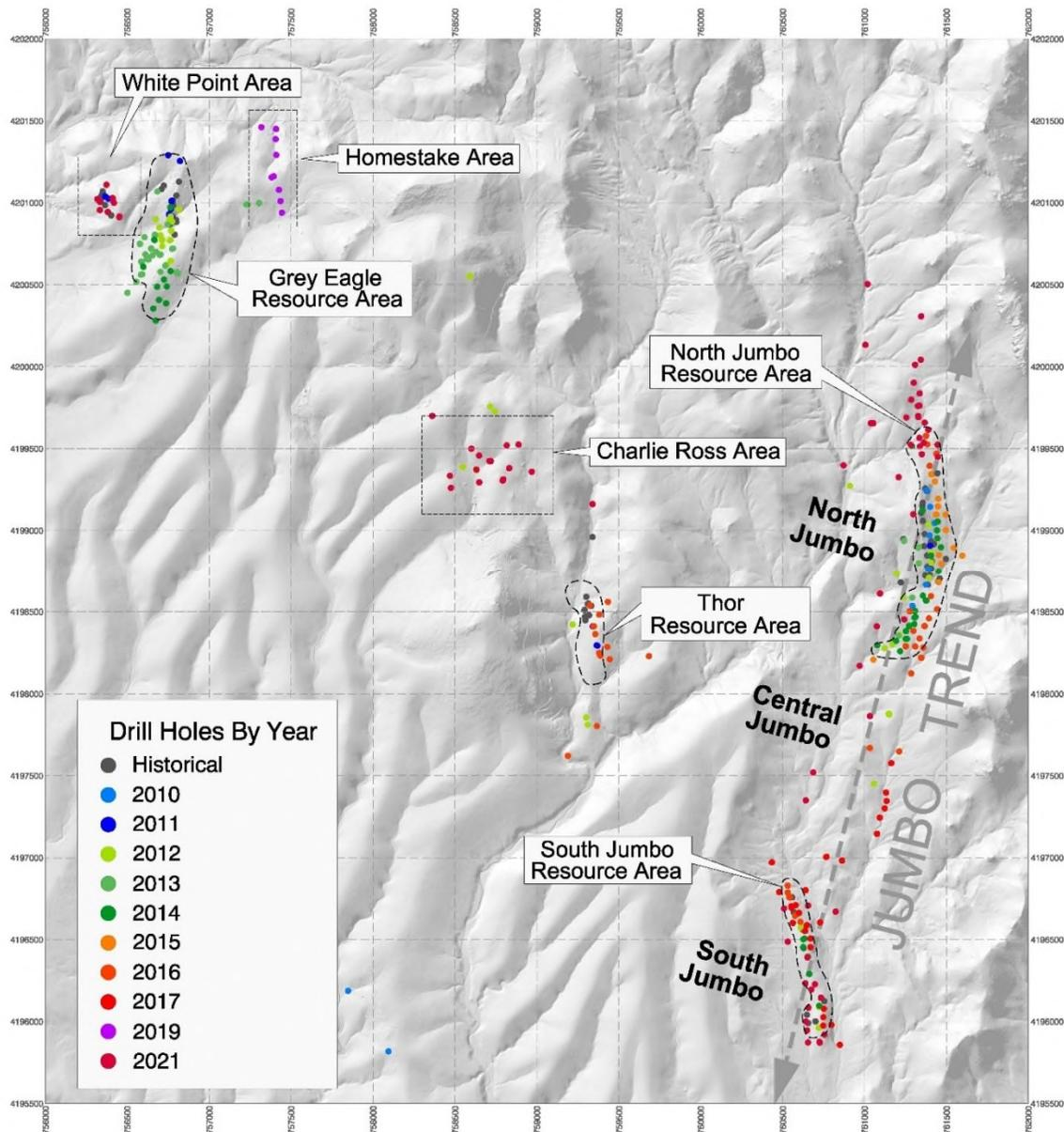
GRC completed a Mineral Resource Estimate and PEA on four of the 33 targets: North Jumbo, South Jumbo, Thor, and Grey Eagle (GRE, 2020). The resource estimate and PEA are based on the assay information from drill holes completed through 2019.
