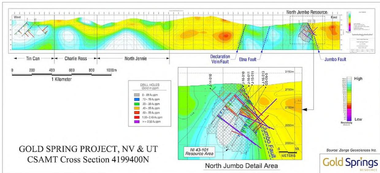
**Figure 9-7: CSAMT Cross Section through North Jumbo-North Jennie**
