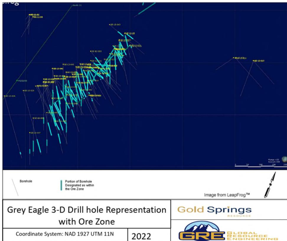
**Figure 14-58: 3-D Representation of the Mineralization Zone Modeling**
