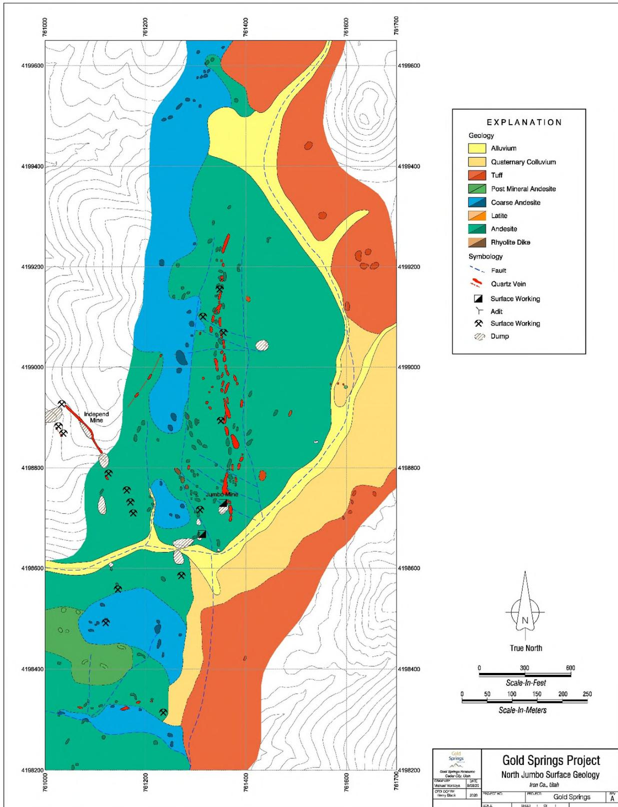
Wallrock alteration surrounding the Jumbo vein system typically extends outward from the vein into the adjacent andesite wallrock up to 200 metres. The low-sulfidation alkaline fluids which formed the main
