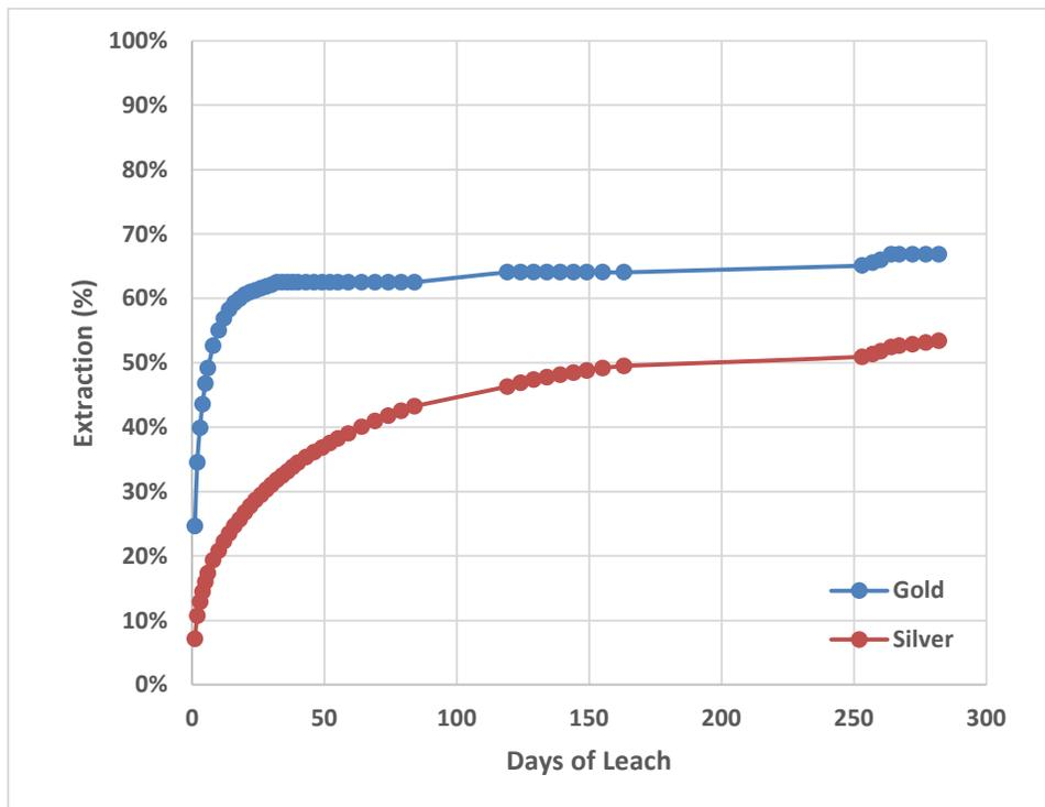
**Figure 13-5 Jumbo Composite 3 Column Leach Results**
