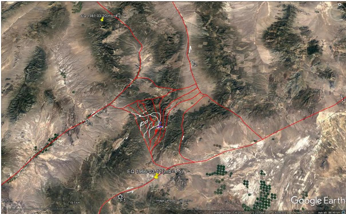
GRE determined the movement mechanism for all above-mentioned faults from satellite images based on morphology and morphotectonic features. They were determined by consideration of sharp and clear displacement of rivers and S-shapes and rhomboidal forms of some drainages. The above-mentioned features are easily defined within the North Jumbo, South Jumbo, South Grey Eagle, and Western F1 faults.
