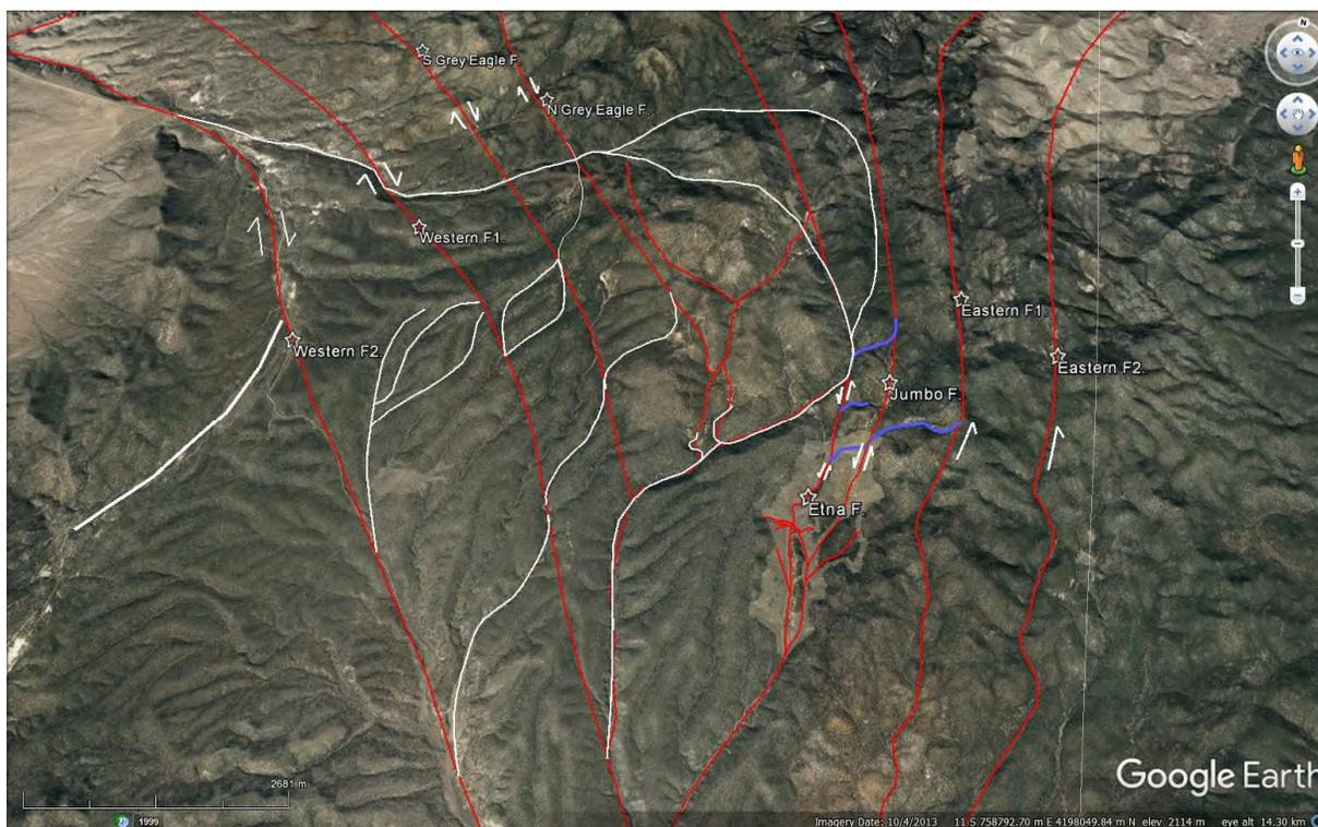
The caldera collapse event lead to increased vertical and downward forces, which may have increased the presence of hydrothermal solution regions in or around the collapsed caldera. As previously mentioned, eight strike slip faults are located in the vicinity of the collapsed caldera, and some of them pass through and cut the caldera. These lineament features and the area between them are important places for hydrothermal activity and mineralization.
