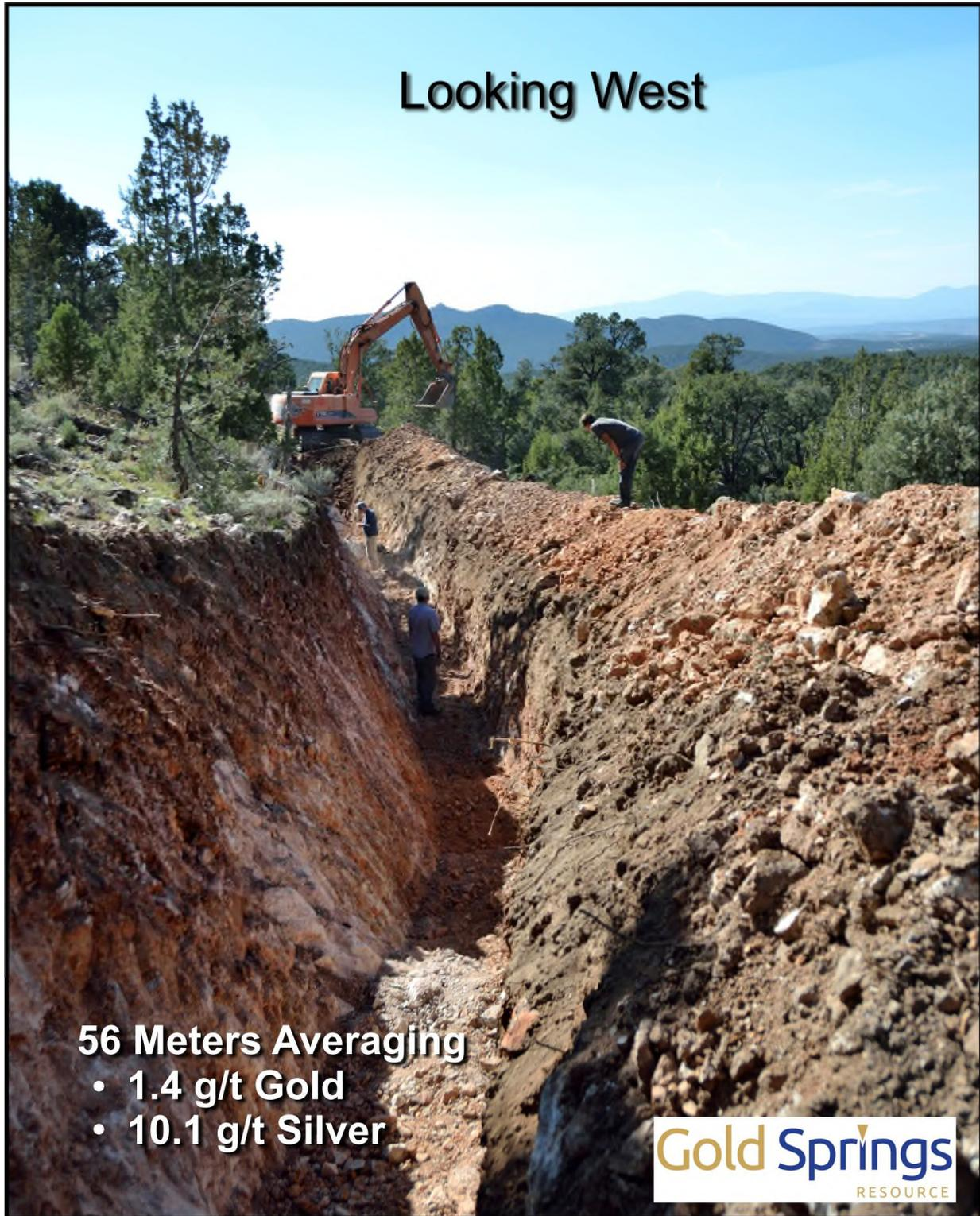
GRC trench through the southern Grey Eagle target area, showing vein mineralization
