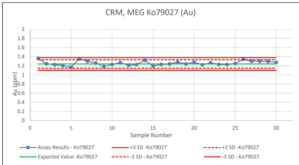
In general, CRMs show reasonable analytical accuracy but relatively poor precision when compared against the certified standard deviation. This poor precision occurs in a number of CRMs from two laboratories for 2021 drilling programs. At this time, it is not possible to definitely determine the cause of CRM high failure rate.
