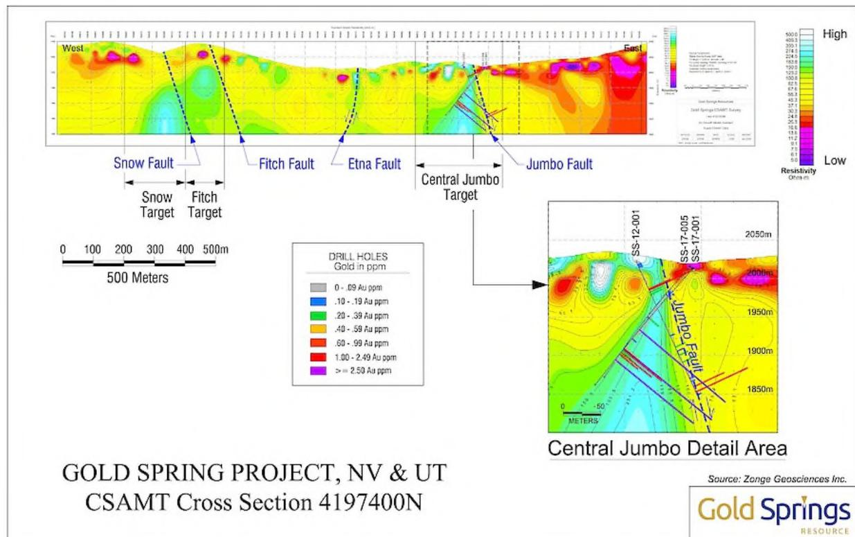
**Figure 9-10: CSAMT Cross Section through Juniper**
