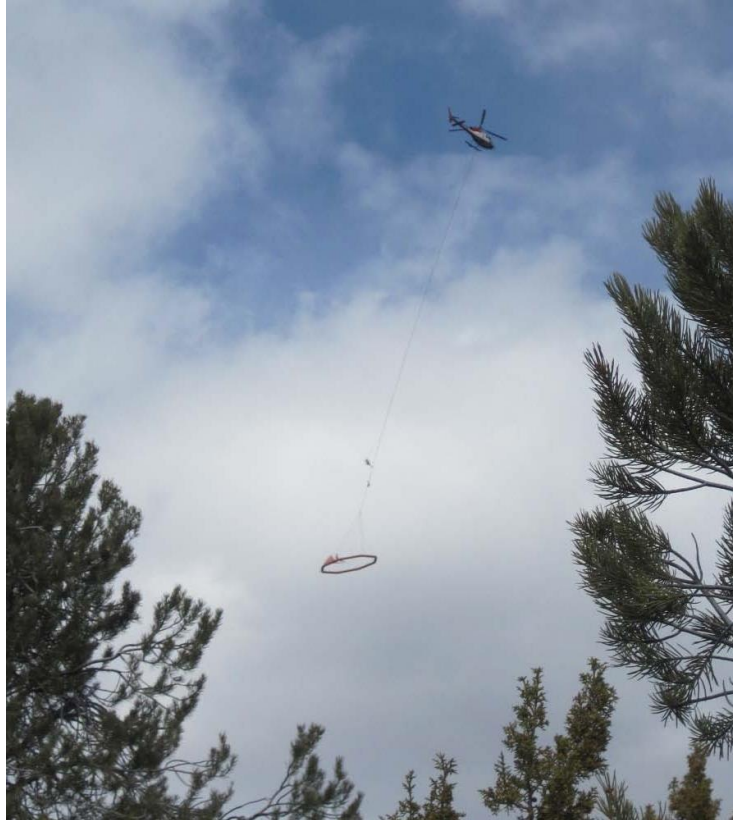
Photo 9-1: Helicopter Conducting ZTEM Survey for GSLLC during 2011
