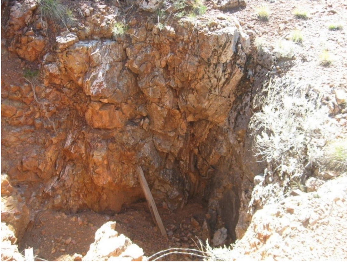
Sample KK-11-39 was collected across 2 metres of this structure Vein exposed in caved stope at the Thor Mine, assays 3.1 g/t gold across the 2 metres face shown above.
