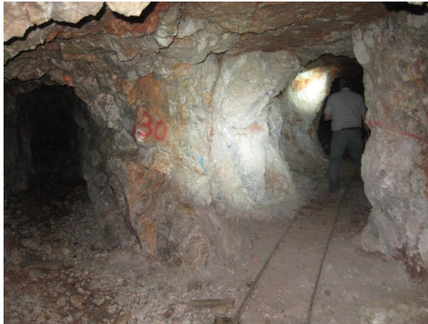
Underground workings in the Grey Eagle area, approximately underneath the GSLLC trench, showing some of the previous Energyx sampling intervals
