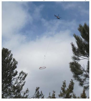
Photo 9-1: Helicopter Conducting ZTEM Survey for GRC during 2011
